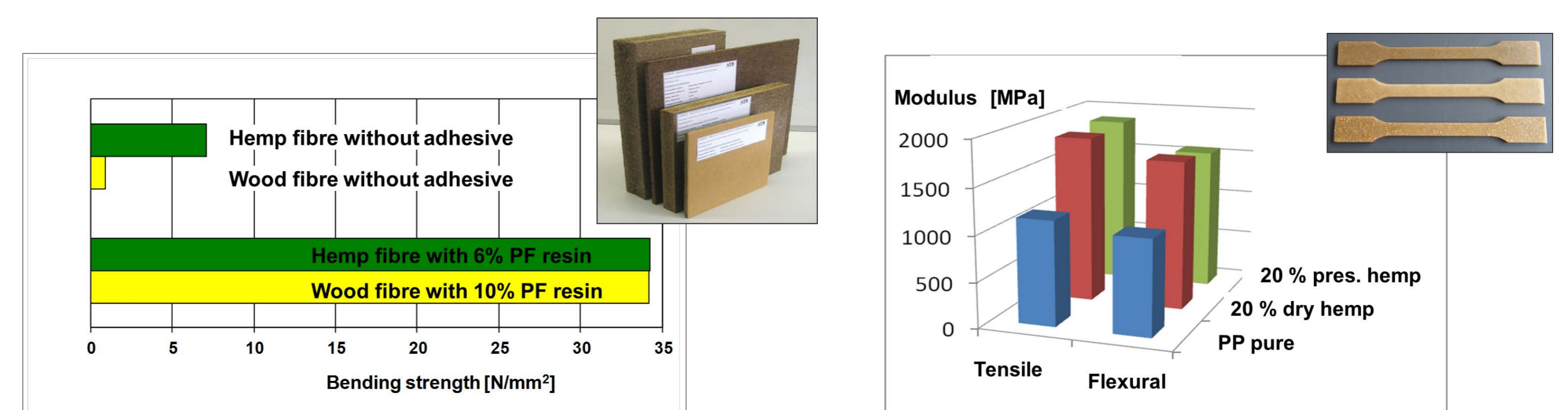
Figure 4 Selected results from the processing of wet preserved hemp into fibre boards (left) and reinforced composites (right)
